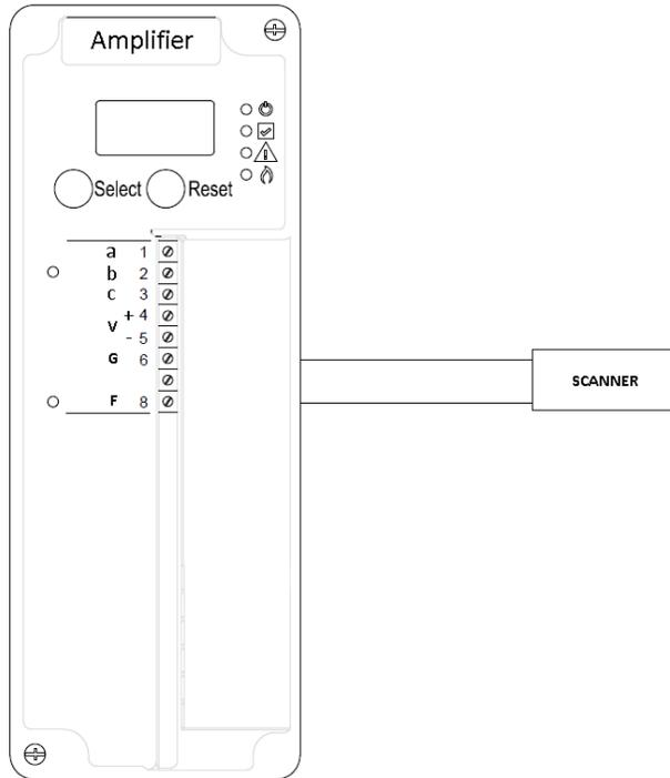
Refer to Installation Instructions for exact wiring of the scanner used on your project. The Lead Lag example uses the UV/Visible Ampli-Check Amplifier Module and scanner. Make sure to change the configuration on your project to match the amplifier/scanner you will use on your project.
