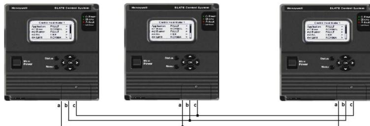
Continuing with the example, let's assume that SLATE device 2 has the sensor value and SLATE device 1 needs the value to control the demand (see wire sheet above).
