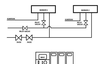
The dual-amplifier approach requires Burner Module configuration to support the feature as well as an additional physical setting on the Amplifier Module.
